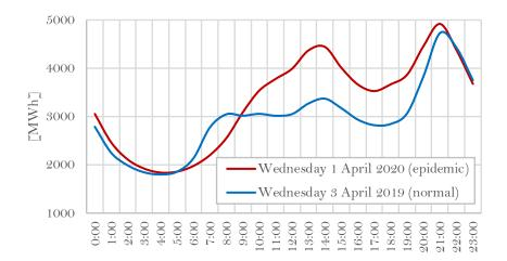
Figure 3. Load profiles for households enrolled in the PVPC and comparison between 2019 and 2020; data from esios [38]
